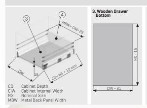
Calculation Method for Front Panel Dimensions:Cut Measurement=Cabinet Internal Width - 99 Calculation Method for Front Panel Dimensions: Cut Measurement=Cabinet Internal Width - 53
