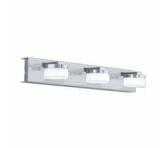
wall light steel, chrome, / plastic, clear, satined / Article Length (in mm): 450, Article Overhang (in mm): 125, Article Height (in mm): 70 LED, 3X7,2W, Lumen Complete: 1710, IP44 Single-Box Height (in mm): 485 Single-Box Length (in mm): 135 Single-Box Depth (in mm): 85
